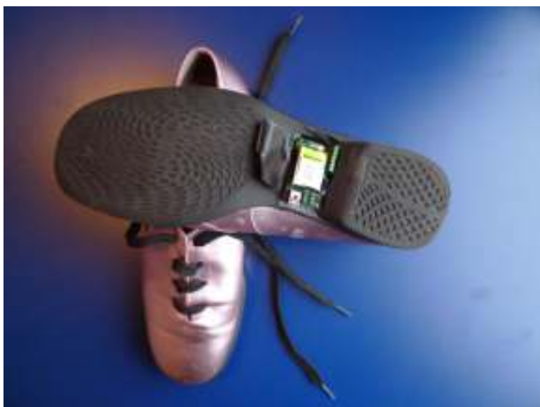
Sensors on the soles of her shoes: Terri Hrons kontrollersko. Foto: Hans Wilmers.
